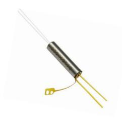
The MOAP MEMS Variable Optical Attenuator (VOA) uses a vibration-insensitive thermal-MEMS mechanism for reliable operation under shock and high-vibration conditions, engineered for aircraft, shipboard, and other vibration-prone platforms. An optional Input Optical Power Monitor integrates an InGaAs PIN photodiode with the VOA in a single hybrid module, reducing component count, and footprint. The VOA exhibits little wavelength dependence and minimal temperature dependence and drift.
